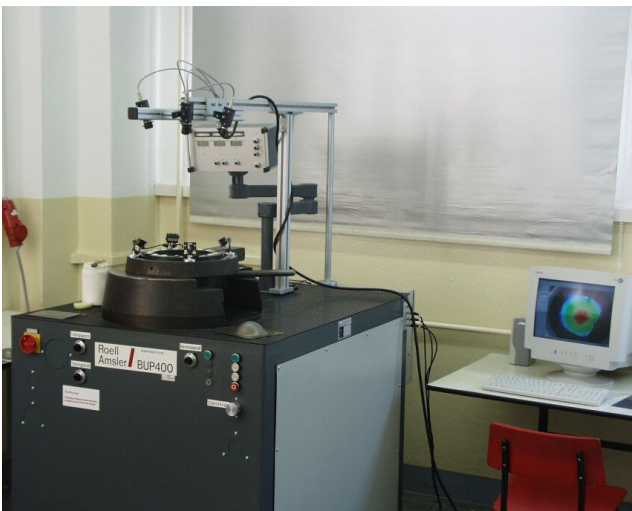
Figure 4: The AutoGrid ® vario system working with a sheet metal testing machine of Roell/Amsler
