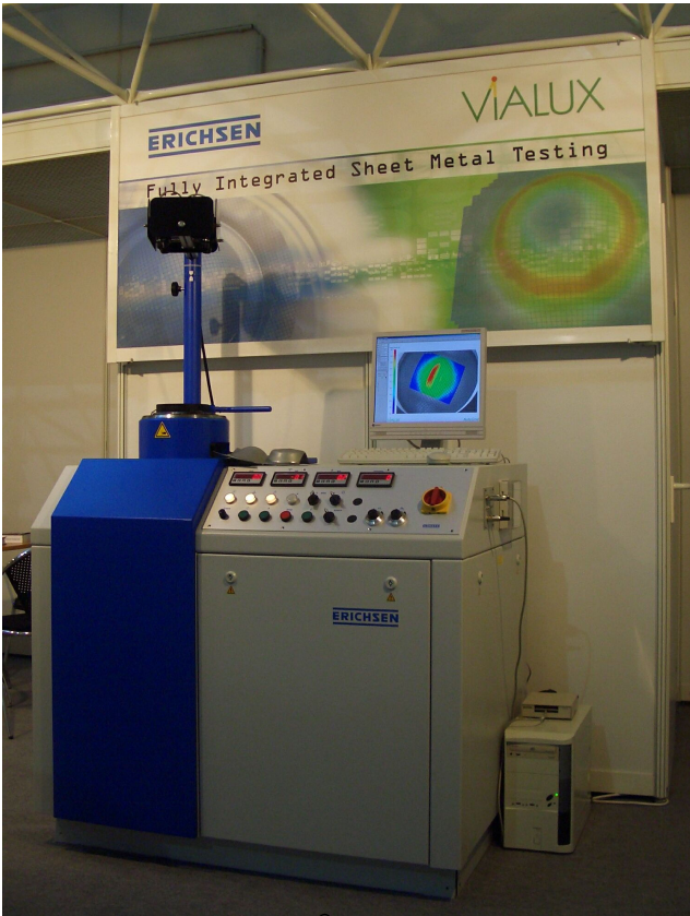
Figure 3: The AutoGrid ® vario system and the sheet metal testing machine of Erichsen comp. as an integrated solution on the EuroBLECH 2004 show
