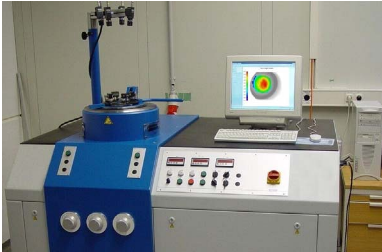
Figure 1. AutoGrid ® vario system for FLC determination at BMW in Dingolfing
