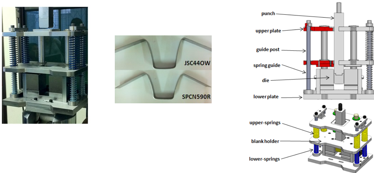
Figure 3 The components of U-bending dies, specimen and the installation in the tensile testing machine
