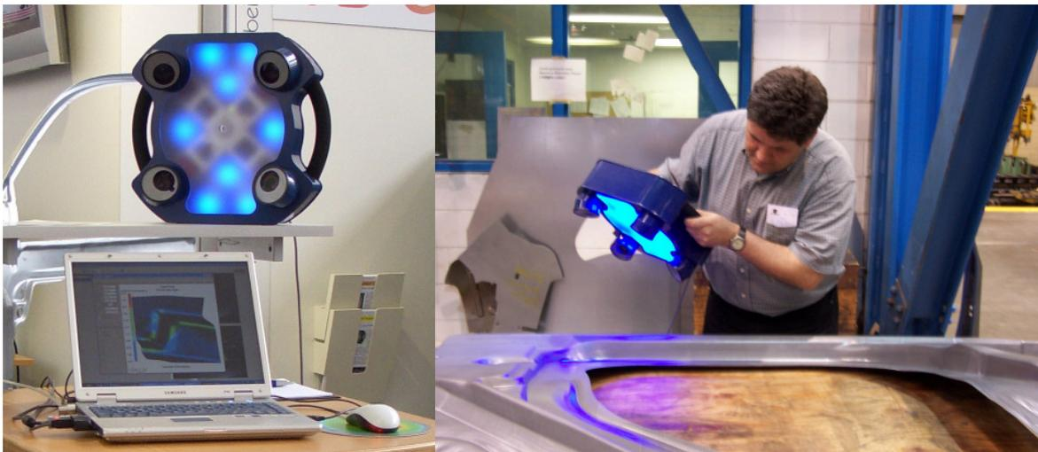
**Figure 6.** The *AutoGrid<sup>®</sup> compact* device connected to a laptop and in action with operator
