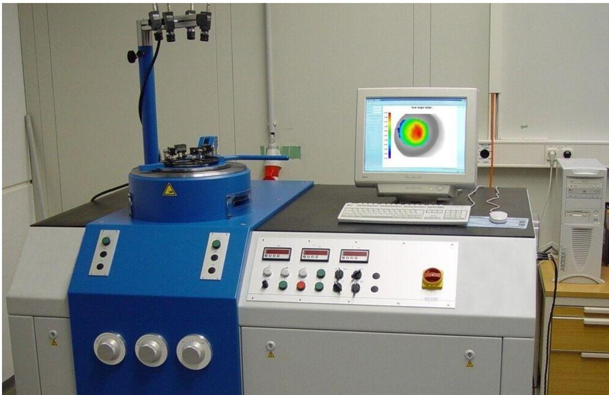
*Figure 1. Strain analysis system AutoGrid<sup>®</sup> integrated into ERICHSEN testing machine for FLC tests*
